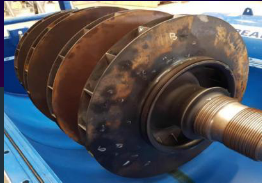
Compressor rotor failure
