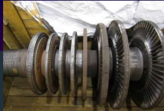
Turbine blades failure
